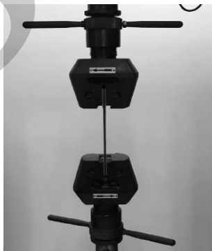
图 7 接头剪切试验装置 Fig. 7 Device of the joint shear test
