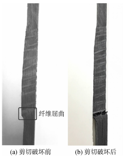
图 20 Z-pin 体积分数为 3.0% 的接头样貌 Fig. 20 Joint appearance of Z-pin volume fraction of 3.0%
